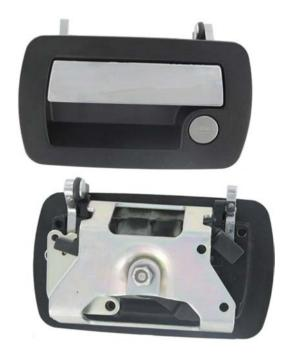
This flush mounted paddle is a redesign of our 030-0450 paddle handle for compartment doors and entrance doors on recreational and specialty vehicles. Containing the same proven mechanical details as previous with a modernized look, it can be used in FMVSS 206 applications, is power lockable and features 2-point remote pivot plate and lock cam actuation.
