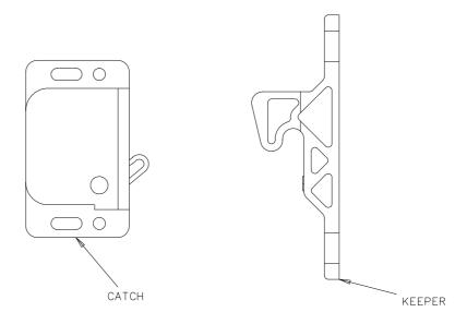
HOLDING FORCE - THE FORCE EXERTED BY THE CATCH ASSEMBLY TO HOLD THE DOOR CLOSED.
